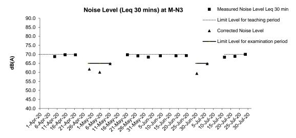
Remark: Corrected Noise Level was applied on 29 April 2020, 5, 11 May 2020, 30 June 2020 and 6 July 2020; Corrected Noise Level = 10\* log(10^(Measured Noise Level/10)) – 10^(Baseline Noise Level/10))
